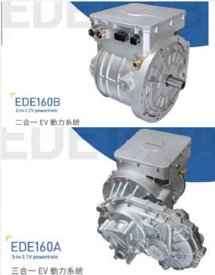
Our in-house developed energy-saving technology EV power system features a highly integrated (3-in-1) drive controller, motor, and gearbox. The characteristics of this design reduce volume and weight, and provide high power density (4.30 kW/liter) power output, low idle loss: close to 0% (fuel vehicle: 3%), high transmission efficiency: 77% to 82% (fuel vehicle: 16% to 25%), zero emission pollution: 0% (fuel vehicle: CO<sub>x</sub>, NO<sub>x</sub>, SO<sub>x</sub>).
