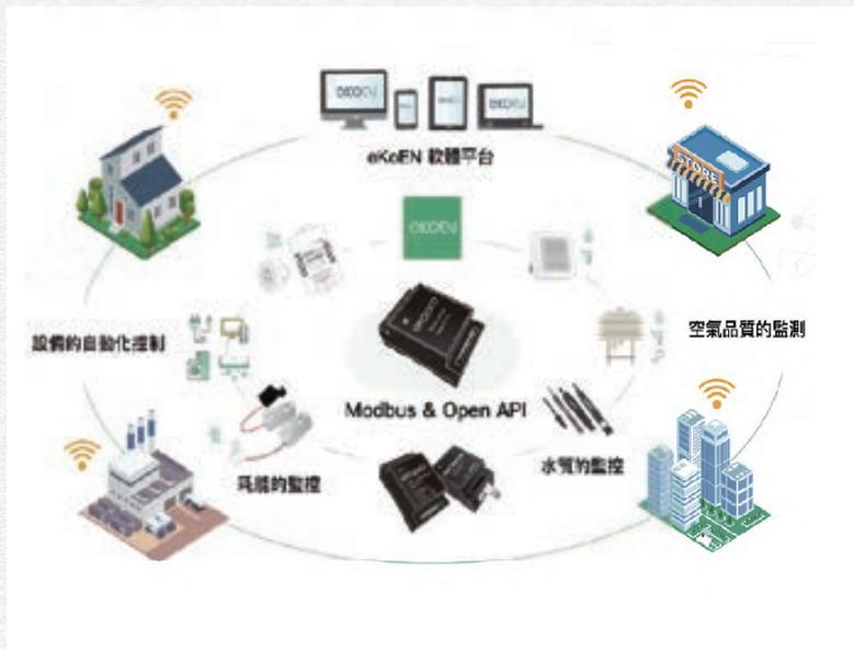
eKoEN is a lightweight energy management system developed, that uses non-intrusive and easy-to-install miniature sensors to collect power data from feeder lines. It can be installed inside the distribution panel without powering off. Compared to most electricity meters on the market, its installation time and cost are reduced by about 15%, making it suitable for small and medium-sized power users to conduct on-site power distribution checks.
